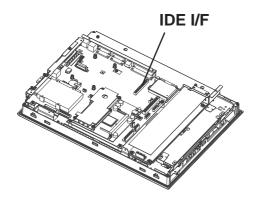
3) Insert the HDD unit's cable connector completely into the IDE I/F.
